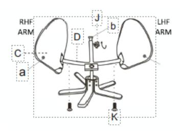
Please ensure that the holes (A) for the backrest fitting are at he rear of the base and opposite the adjustment bar (B). Do not tighten screws until product is fully assembled.
